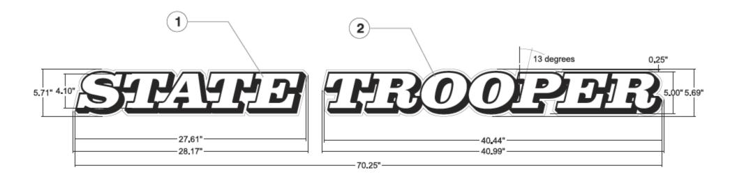
NOTE: Decal to have Vehicle Side and Position stamped on premask
